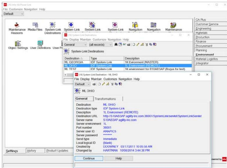
System Link must be installed and activated in all environments. System-Link Destinations must be set up on the Environment application card of XA. The information set up on a system-link destination must be consistent among all the environments. In order to pass MRP planned demand, the Transformation – Replicate\_TransferDemandForCommonLoad must be activated.
