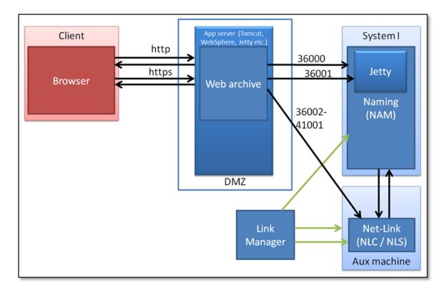
The web components of Net-Link run in a Servlet container. Examples of such a container are Apache Tomcat and IBM WebSphere. The components are packaged into a Web Archive (WAR)file.
