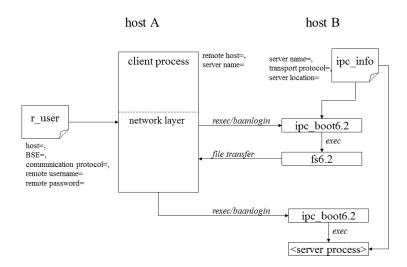
On the remote host, the ipc boot process retrieves from the ipc info file (\$BSE/lib/ipc info) the path of the fs executable, as well as the transport protocol. That information overwrites the ipc boot process with an fs process. The fs is the Enterprise Server internal file server that enables remote file access.
