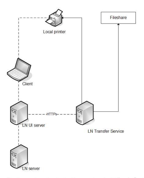
The diagram shows the typical architecture, where the LN Transfer Service is installed on a separate print server. This print server is connected, through HTTPS, to the LN UI server. The LN Transfer Service can print to a local printer or to a file share.
