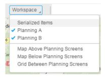
The Serialized items, Planning A and Planning B are the various sections in the workbench. The toggle menu and the docking control, allows you to minimize or maximize these sections.
