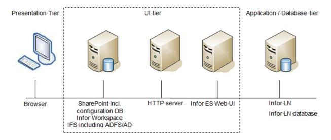
For smaller configurations, you can install a separate HTTP server and the Web application server on the same physical server.
