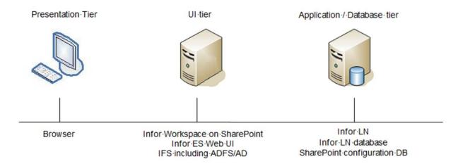
In this scenario the UI components are stored in a single UI tier, and the application and database components are stored on another tier. This configuration is recommended for small installations.
