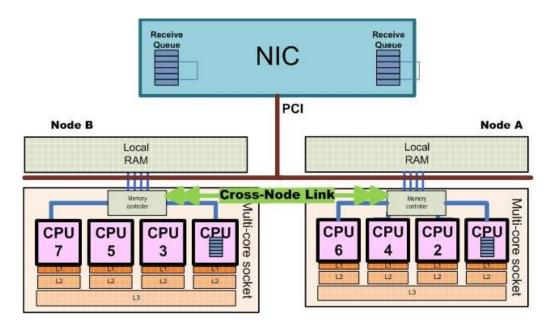
In principle, a NUMA based system is split into nodes, with a NUMA-node for each Multi-core socket. This means that the system memory is also divided across the nodes. Local memory can be quickly accessed but memory on other node(s) must be accessed using the cross-node link with more latency.
