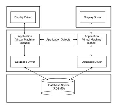
In this second configuration, the application tier is placed on one server, while the database driver and database server are placed on another. As with the previous configuration, an instance of the application virtual machine and at least one instance of the database driver is started for each user. All users have access to the same application objects and database servers.
