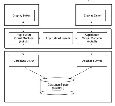
Many other configurations of client/server systems are available, including dividing the application logic among multiple servers or using multiple servers to distribute the database.
