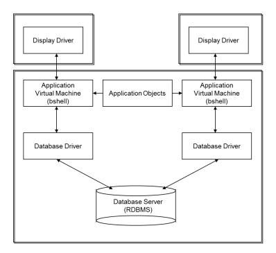
If two machines are to be used as servers, two configurations are commonly used. In both configurations, the display drivers reside on the user workstations.
