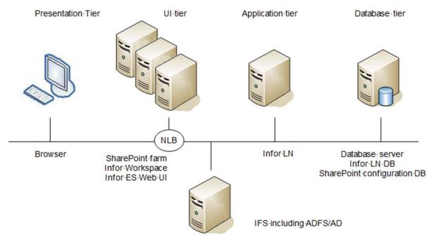
**Note:** IFS is installed on a single server. You can have only one instance of IFS and the SharePoint configuration DB.
