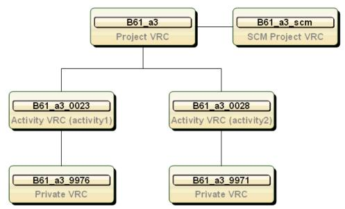
This diagram shows the VRC structure after an intermediate code freeze.
