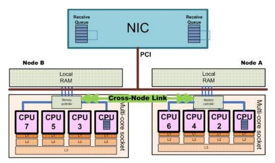
In principle a NUMA based system is broken up in nodes, with in most cases a NUMA-node for each Multi-core socket. This means that the system memory is divided over the nodes as well. Local memory can be accessed fast but memory on other node(s) has to be accessed by the cross-node link and has more latency with a bigger chance of contention.
