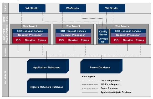
**Note:** The above diagram applies to environments with multiple web servers. In environments with just one web server (the utility server typically serves as a web server), only "Web Server x" would be used.
