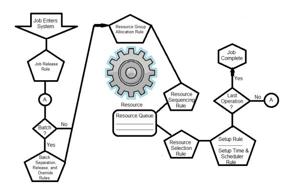
The Scheduler provides you with a wide variety of logic to use for modeling your manufacturing facility. This logic should cover the manufacturing system you will be modeling with this system. However, you might find that your facility contains some unique situations that require special logic to model them accurately.
