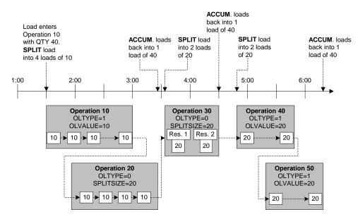
1 The processing at operations 10 and 20 proceeds the same as with the previous overlapping operations example. Note that the SPLITSIZE parameter is defined in operation 20; the Scheduler ignores it because the operation is overlapped.
