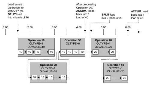
The diagram below illustrates a typical overlapping operation situation.
