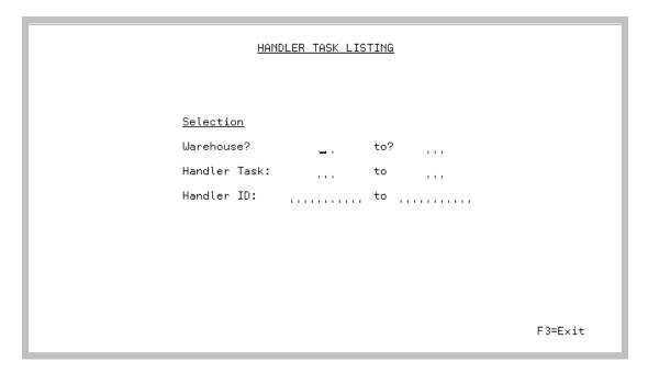
This screen displays after selecting option 12 - Handler Tasks Listing (MENU RFFILE). Use this screen to determine which handler tasks will print on the listing.
