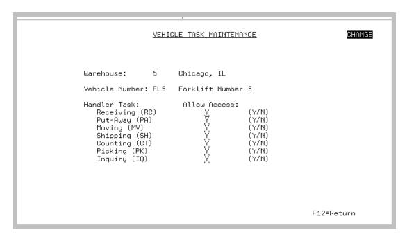
This screen appears after pressing ENTER on the Vehicle Task Maintenance Selection Screen (p. 12-3), if the **User Task** field blank. Use this screen to provide or restrict performance of system-defined tasks by the displayed vehicle for the indicated warehouse.
