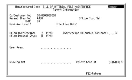
This screen displays after selecting a function, type of bill of material, and parent item number on the Bill of Material File Maintenance Selection Screen (p. 9-5). Use this screen to specify information for the parent item in the bill of material.
