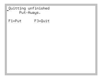
The Quit Unfinished Put-Aways Screen displays after pressing F3=Return on the System Put-Away Number Verification Screen (p. 3-22) with outstanding put-away transactions assigned to the handler. Use this screen to return to complete the put-away transactions or cancel the remaining put-away transactions.
