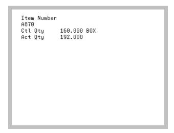
The Pallet Control Exception Screen appears after pressing F1=AUTO PA from the Receiver Identification Screen (p. 2-5) when the pallet control quantity to be received is different than the actual quantity received for a pallet control item in the selected receiver.
