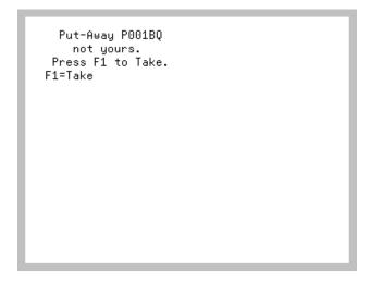
The Take Put-Away Assignment Screen displays after entering a put-away number on the Manual Put-Away Number Identification Screen (p. 3-5) or the System Put-Away Number Identification Screen (p. 3-18) that has been assigned to another handler. Use this screen to take the put-away assignment from the original handler and complete the put-away tasks.
