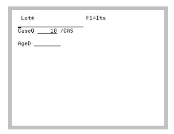
The Lot Number Identification Screen only displays if receiving lot control items and a 2=Prompt, not required or 3=Prompt, required was entered in the Receiving: Lot/Serial Prompt Option field on the Task Options Maintenance Screen in Radio Frequency Options Maintenance (MENU RFFILE).
