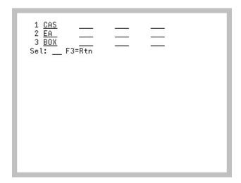
The U/M List Screen appears after you press F2=U/M LIST on the Item Cross Reference Screen (p. 1-24). Use this screen to select a valid stocking or alternate unit of measure for the item for which you are adding a cross reference.
