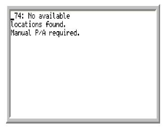
The Radio Frequency Put-Away Message Screen displays from various put-away screens. Some messages are informational, some are warning messages, and some require action by the handler. Use this screen to read and complete the appropriate action based on the specific message.
