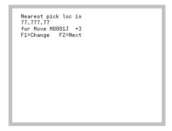
The Move Nearest Pick Location Screen displays when you press F2=NEXT on the Pick Location Identification Screen (p. 4-10) or the Move Number From Location Identification Screen (p. 4-15). Use this screen to review the nearest location for the next move. Or use one of the function keys to manually change the pick-from location or select to skip this location and present the next location using the travel path based on the picking sequence number.
