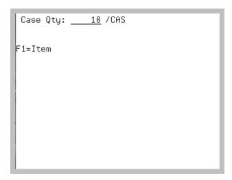
The Count Lot Variable Case Quantity Screen displays after entering lot numbers on the Count Lot Number Identification Screen (p. 7-25) for a lot item that requires verification of the variable case quantity, as defined in Item Balance Maintenance (MENU IAFILE). Use this screen to enter the variable case quantity for the cases being counted.
