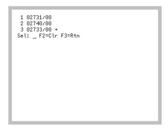
The Selected Orders/Containers List Screen displays after the pressing F1=LsT on the Picking Section Selection Screen (p. 8-5). Use this screen to display the list of orders/containers you have selected for picking, or to delete orders/containers from this list.
