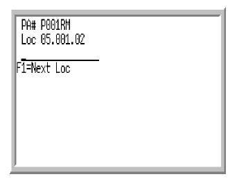
The Put-Away Location Screen displays after scanning/keying at least one valid put-away number and pressing Enter twice or F1=Store on the System Put-Away Number Identification Screen (p. 3-18) or pressing F1=Next Loc from the System Put-Away Number Verification Screen (p. 3-22). Based on the selected put-away numbers and the put-away sequence numbers assigned to the locations, the handler is directed to the first location for this series of tasks.
