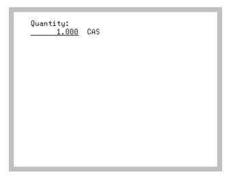
The Move To Quantity Screen displays after pressing ENTER or F3=RETURN on either the Move To Location Screen (p. 4-50), the Move To Lot Number Screen (p. 4-55), or the Move To COO Screen (p. 4-57). Use this screen to enter the quantity of items for storage.
