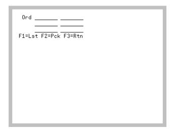
The Pick Order/Container Select Screen displays after the second time ENTER is pressed on the Picking Section Selection Screen (p. 8-5) when the **Scn LbI** field is O or C. when **Pick From Multiple Pick Sections** is set to N through Radio Frequency Option Maintenance (MENU RFFILE).
