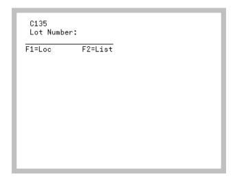
The Move To Lot Number Screen displays after scanning/keying an item number for a lot item and pressing ENTER on the Move To Location Screen (p. 4-50). Use this screen to scan/key the lot number of the item being stored in the location.
