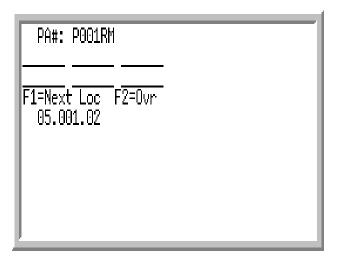
The System Put-Away Number Verification Screen displays after pressing ENTER on the Put-Away Location Screen (p. 3-20). The first 2 put-aways for this location will display. If some or all items cannot be put-away at this location, you may use F2=OVR to override the suggested location.
