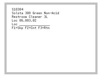
The Picking Location Screen displays after press ENTER on the Picking Summary Screen (p. 8-18). This screen will display the item number and item descriptions and the location within the picking section for you to pick from. If you entered a picking section starting and ending location on the Picking Section Screen (p. 8-5), only a location within those parameters will be shown.
