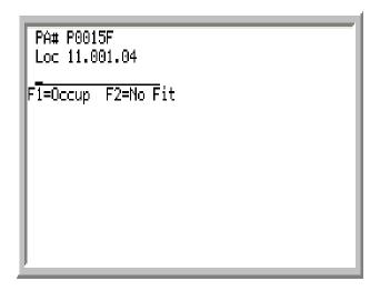
The Manual Put-Away Location Identification Screen displays after entering a valid put-away number and pressing ENTER on the Manual Put-Away Number Identification Screen (p. 3-5). This screen displays the selected put-away and its corresponding assigned location. Use this screen to either confirm the put-away location for the selected put-away or to perform a manual override for the assigned location.
