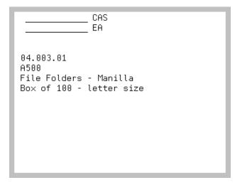
The Count Quantity Screen displays after pressing F1=CNT on the Inquiry Item Information Screen (p. 6-12) or after selecting a location in the **Sel** field and pressing F1=CNT from the Item/Location Location Selection Screen (p. 6-6) for regular items. It also displays from the Case Quantity Value Entry Screen (p. 6-35) and the Lot Expiration Date Entry Screen (p. 6-36) after pressing ENTER.
