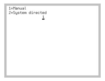
The Put-Away Method Selection Screen displays after selecting F2=PUT and pressing ENTER on the Task Selection Screen (p. 1-8). Use this screen to select the method of putting away inventory after receiving it. You can select either the manual or the system-directed process of putting away inventory.
