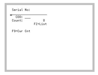
The Count Serial Number Identification Screen displays after keying/scanning a standard serial item (**WH Mgmt Code** is **S**) on the Count Item Identification Screen (p. 7-11). Use this screen to record the serial numbers of count items.
