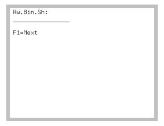
The Count Location Identification Screen displays after pressing ENTER on the Count Type Selection Screen (p. 7-4) or the Count Unit of Measure Quantities Screen (p. 7-18) with the last location completed displayed for reference.
