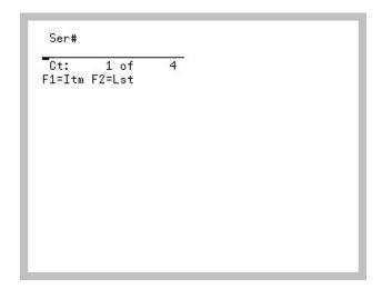
The Serial Number Identification Screen displays after entering quantities on the Quantity Identification Screen (p. 2-29) for a serial item. Use this screen to scan/key the serial numbers of the received items.
