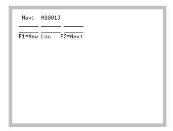
The Move To Number Identification Screen displays after pressing ENTER on the Store Location Identification Screen (p. 4-20), or the Move Nearest Store Location Screen (p. 4-22). Use this screen to enter the number of the move you are storing.
