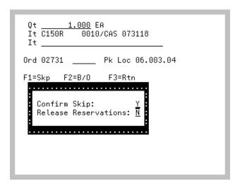
The Confirm Skip and Release Reservation Message Screen appears as a pop-up window after pressing F1=SKP on the Picking Location Screen (p. 8-23), Pick Case Confirmation Screen (p. 8-39) or the Pick Confirmation Screen (p. 8-31), when the **Confirm F1=Skp** option is set to **Y** and the **Allow override of reservation release on F1=Skp** is set to **Y** in Radio Frequency Options Maintenance (MENU RFFILE) for the warehouse.
