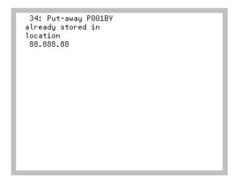
The Put-Away Already Stored in Location Screen displays after entering a put-away number on the Manual Put-Away Number Identification Screen (p. 3-5) or the System Put-Away Number Identification Screen (p. 3-18) that has already been stored and completed. Use this screen to verify the scanned/keyed put-away number. If the put-away number scanned/keyed is correct, follow warehouse business practices for the discrepancy.
