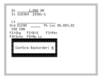
The Back Order Confirmation Screen appears as a pop-up window after pressing F2=B/O on the Pick Case Confirmation Screen (p. 8-39) or the Pick Confirmation Screen (p. 8-31), when the **Confirm F2=B/O** option is set to Y in Radio Frequency Options Maintenance (MENU RFFILE) for the warehouse.
