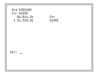
The Stage Location List Screen appears after pressing F1=STGD LST on the Interim to Stage Screen (p. 8-55), the Interim to Dock/Stage to Dock Screen (p. 8-60) or the Stage to Dock Screen (p. 5-9). This screen lists the other staging locations that are storing inventory for the order. Use this screen to select an alternate staging location for the inventory in the interim location.
