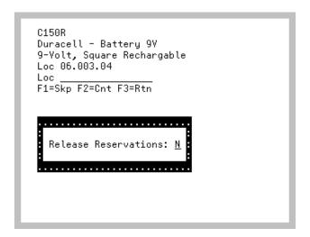
The Release Reservation Message Screen appears as a pop-up window after pressing F1=SKP on the Picking Location Screen (p. 8-23), Pick Case Confirmation Screen (p. 8-39) or the Pick Confirmation Screen (p. 8-31), when the **Confirm F1=Skp** option is set to N and the **Allow override of reservation release on F1=Skp** is set to Y in Radio Frequency Options Maintenance (MENU RFFILE) for the warehouse.
