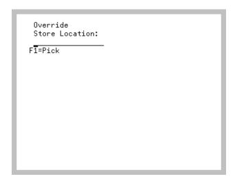
The Move Queue Override Store Location Screen appears after pressing F7=OVR STORE LOC on the Move Queue Pick Location Screen (p. 4-71). During this RF move queue process, you will be able to place inventory into an override store location. This override store location will take all moves that have been picked by the handler and have not yet been completed, and then place these moves into the override store location specified by the handler.
