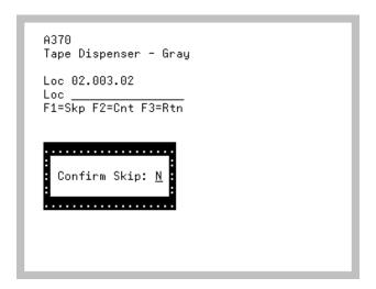
The Confirm Skip Message Screen appears as a pop-up window after pressing F1=SkP on the Picking Location Screen (p. 8-23), Pick Confirmation Screen (p. 8-31), or the Pick Case Confirmation Screen (p. 8-39) when the **Confirm F1=Skp** option is set to Y and the **Allow override of reservation release on F1=Skp** is set to N in Radio Frequency Options Maintenance (MENU RFFILE) for the warehouse.
