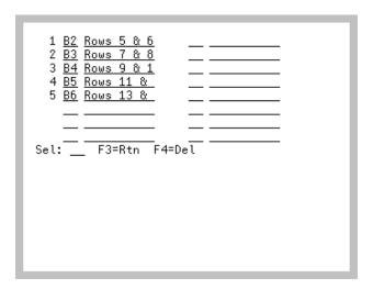
This screen displays after pressing F9=LsT on the Picking Section Selection Screen (p. 8-5). Use this screen to view a list of the selected picking sections where the handler will work. This screen is also used to remove picking sections from the list.
