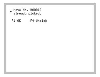
The Move Number Already Picked Screen displays after pressing ENTER on the Move Number From Location Identification Screen (p. 4-15), when the move number scanned/keyed has already been picked. Use this screen to accept the message or unpick the move number already picked.
