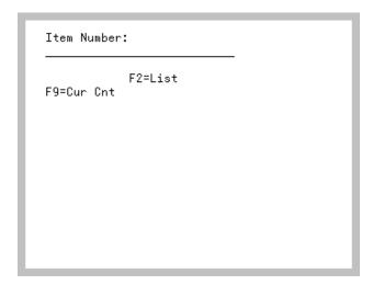
The Count Item Identification Screen displays after scanning/keying a location and pressing ENTER on the Count Location Identification Screen (p. 7-6). Use this screen to identify the items you plan to count in the selected location.
