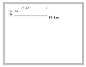
NOTE: If the item you are picking is a T-type tracked serial item, the screen will display three lines for you to enter a serial number on. If the item you are picking is an S-type standard serial item, the screen will display only two lines: one line displaying the requested serial number for you to pick and a second line for you to enter the actual serial number of the item you pick. Serial items are defined as T or S-type in Item Master Maintenance (MENU IAFILE).
