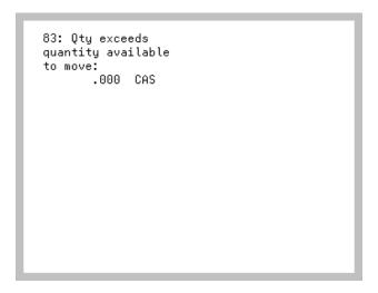
The Quantity Exceeds Available Message Screen displays from Remove From Quantity Screen (p. 4-36) when the quantity entered is larger than the available quantity to move. Use this screen to read and complete the appropriate action based on the specific quantities being reported.
