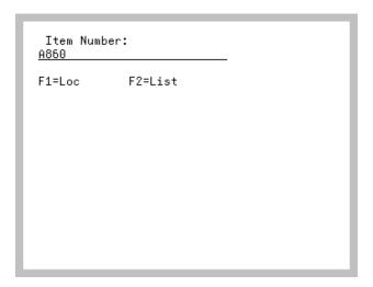
The Remove From Item Number Screen displays after scanning/keying a location and pressing ENTER on the Remove From Location Screen (p. 4-30). Use this screen to scan/key the number of the item you plan to remove from the location.
