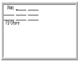
The System Put-Away Number Identification Screen displays after selecting option 2=System Directed to select the system-directed put-away process from the Put-Away Method Selection Screen (p. 3-3). This screen also displays after the selected group of put-away transactions have been completed. The handler will either select another group of put-away numbers or press F3=Return to exit the put-away task.
