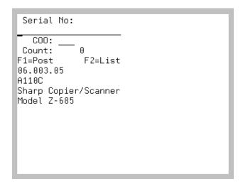
The Count Serial Number Identification Screen displays after selecting a location and pressing F1=CNT for a serial item on the Inquiry Item Information Screen (p. 6-12) or after selecting a location in the **Sel** field and pressing F1=CNT from the Item/Location Location Selection Screen (p. 6-6). Use this screen to record the serial numbers of count items.
