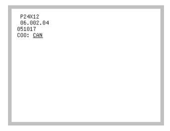
The Remove From COO Screen displays only if you are moving a country of origin tracked item, as determined through Item Master Maintenance (MENU IAFILE), and the item is not a serial type item. For serial type items, the COO is tracked with the serial number on the Remove From Serial Number Screen (p. 4-44).
