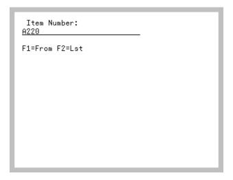
The Move To Item Number Screen displays after removing multiple items from their stored locations and pressing F1=To from the Remove From Location Screen (p. 4-30). It also displays after pressing ENTER on the Move To Quantity Screen (p. 4-53), or F1=To on the Remove From Item Number Screen (p. 4-33) if you replenish a location with more than one item number.
